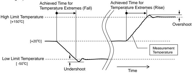
During increasing and decreasing the temperature, the gradient is a little fluctuated on starting and stopping the cooler. (about  $5^{\circ}$ C)
